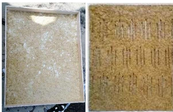
**Gambar 3.** Panel Absorpsi Tanpa Lubang (Kiri), Panel Absorpsi Rongga Halus dan Berlubang (Kanan)
