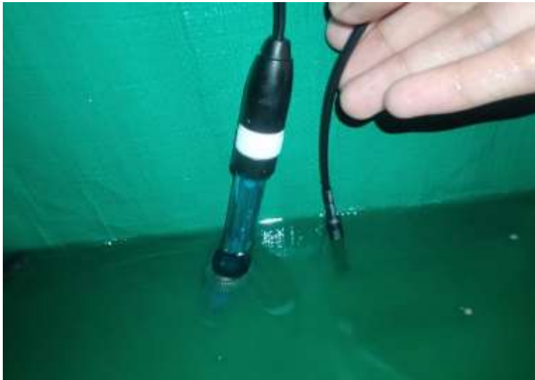
Fig 3.3 Temperature and pH Sensor Testing
