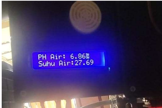
Fig 3.10 Temperature and pH Sensor Testing
