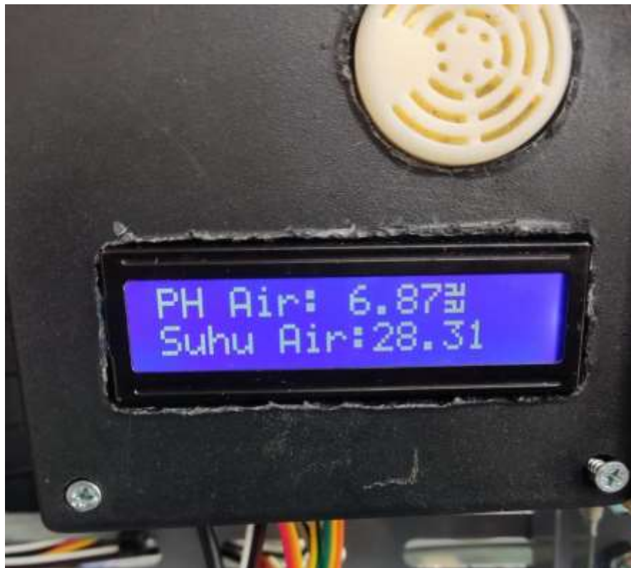
Fig 3.4 Results of reading pH and temperature values
